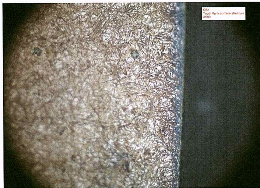
Picture 2: Surface microstructure at tooth flank (X500)
