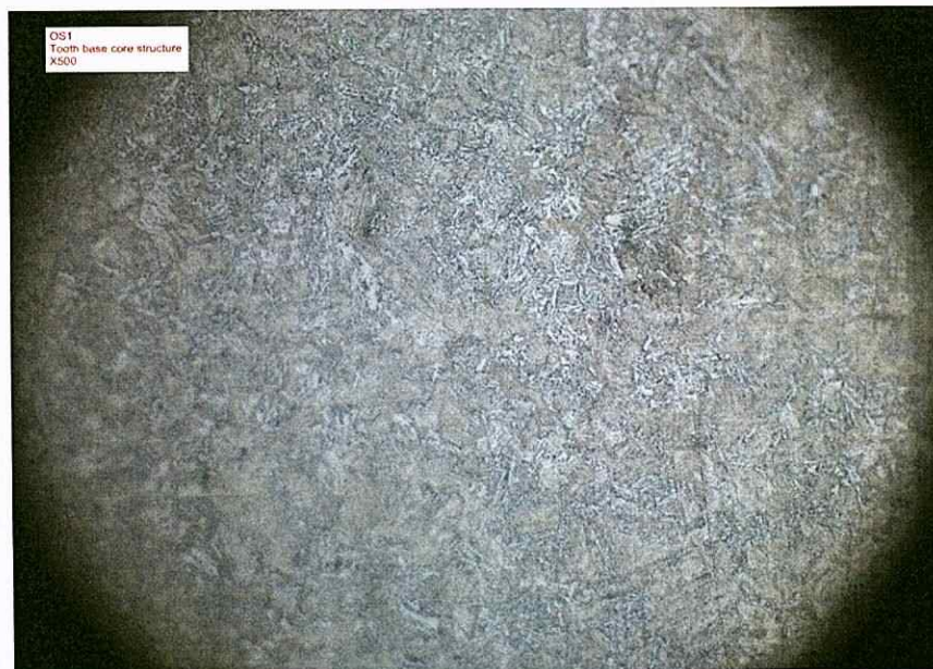
Picture 3: Core microstructure at tooth base (X500)
